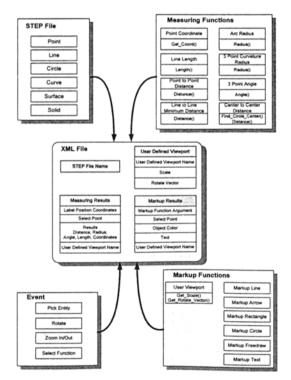
Fig. 6. Architecture of the dimensional verification and markup functions.
