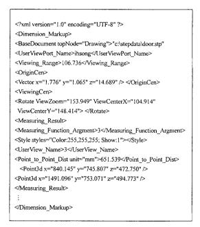
Fig. 8. XML document of markup result for dimensional verification.
