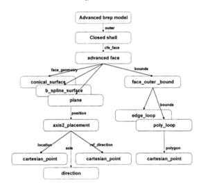
Fig. 4. Structure of the advanced brep model.
