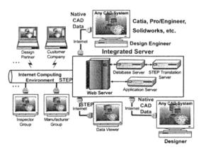
Fig. 1. Structure of the Web-based design and dimension verification system.
