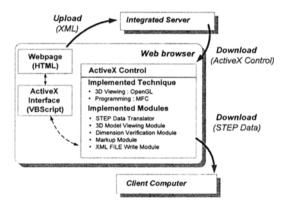
Fig. 2. Configuration of the client ActiveX for CAD data verification.
